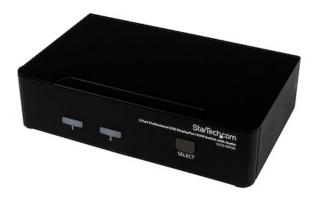
The SV231DPUA 2-Port USB DisplayPort KVM Switch delivers dual computer KVM control, for demanding high definition multimedia applications. Supporting DisplayPort connections with a native resolution of 2560 x 1600, and support for both 7.1 HD digital audio (when connected to supporting displays and sources) and 3.5mm stereo analog audio/mic.
