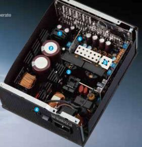
Special heat sink design for 12V switching circuit
