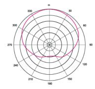
Directivity: Uni-directional Frequency Response: 50Hz - 14 KHz
